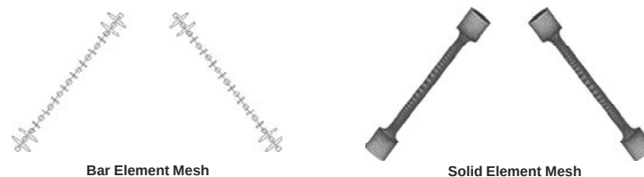
Figure 8.1 FEA beam model (left) and solid element model (right) of bipod flexure.
