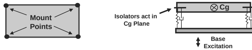
Figure 7.51 Optical bench mounted on four vibration isolators in the plane of the center of gravity of the optical bench.
