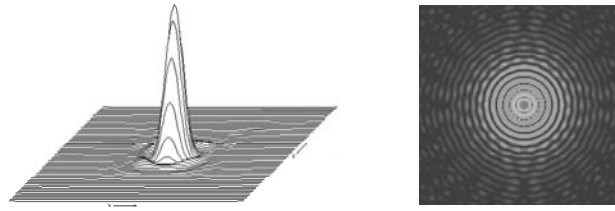
Figure 2.18 PSF for an aberration-free system.
