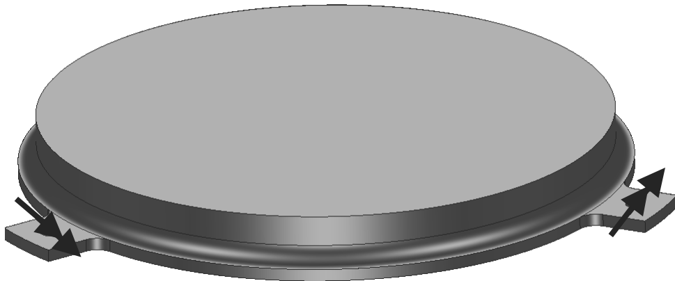
Figure 5.28 Full CAD geometry of a mirror with threefold symmetry.
