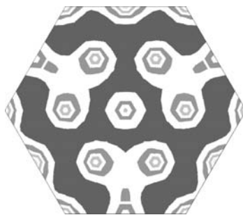
Figure 10.7 Corrected surface deformation for both actuator configurations.
