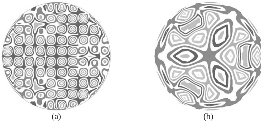
Figure 5.22 Residual surface deformation after all Zernike terms through hexafoil are subtracted: (a) 3D plate/shell model and (b) 3D effective model.
