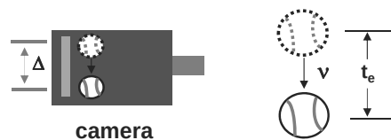
Figure 7.35 Point spread function produced by constant velocity image smear.
