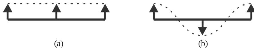
Figure 13.9 Two possible forms of response within the envelope: (a) all-rigid-body motion and (b) all-elastic motion.
