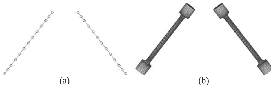
Figure 6.32 Finite element models of example beam flexures: (a) beam model and (b) solid model.
