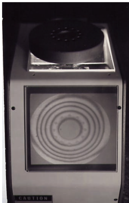
Figure 6.3(b) Acceptable base surface, in which no out-of-plane deformation around the screw holes occurs and good rotary symmetry is achieved.
