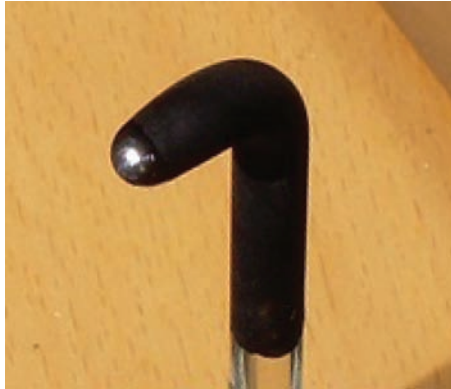
Figure 3.9(d) Molten-glass rod cap for diverging a plain laser beam.
