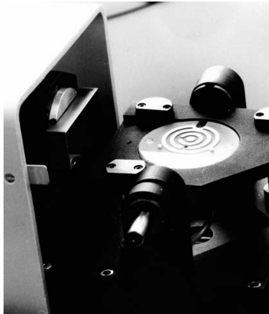
Figure 9.12(a) A chuck with reference zone in a reverting two-beam interferometer (Fig. 9.8). The chuck holder rests on three height-controllable anvils. The wafer-holding chuck area is plane parallel to the reference zone; the height difference between the two plateaus equals the specific proprietary wafer thickness. The reference zone serves in the computer-aided evaluation of thickness and its variation and tilt between the wafer surfaces.
