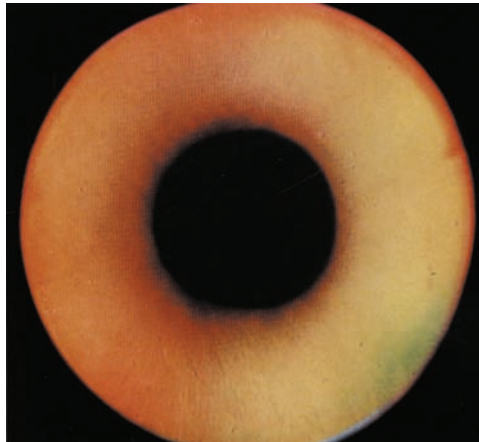
Figure 8.10(b) A micromachined sample at the limit of being acceptable.
