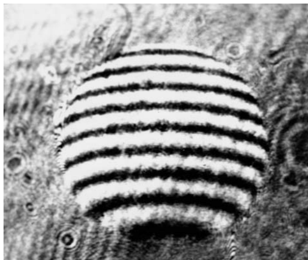
Figure 2.5(b) Spurious coherent reflections and stray light deteriorate the fringe definition. [See the vector diagram uncertainty circle in Fig. 3.2(c).]
