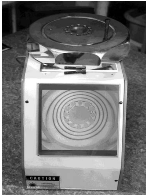
Figure 6.3(a) Unacceptable base surface of a polygon mirror wheel. Connection to the complementary hemisphere of the air-bearing spindle will deform the entire polygon body (reprinted from Ref. 2).
