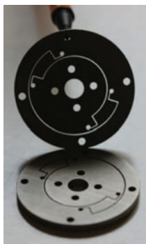
Figure 3.9(b) Homemade XYZ pinhole alignment fixture with fine Z motion by the sleeve gliding on a micro-optics housing with a differential thread.
