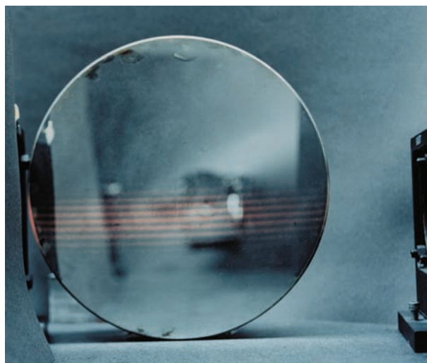
Figure 1.18(c) Due to the double reflection at the mirror and the preset 80 deg of incidence, the Fizeau scatter interference levels represent a mutual distance, as viewed orthogonally on the mirror, with 1 fringe equivalent = 0.913\ \mu\text{m} at the HeNe laser wavelength.
