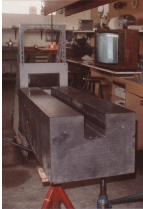
Figure 9.7(a) Granite air-bearing machine bed tested by LIHO during the final lapping. The TV monitor display is shown in Fig. 9.7(b).
