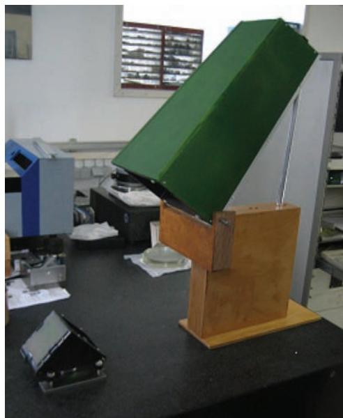
Figure 1.14(c) Collimator with Z-folded beam inclined to suit. The image is seen on a transparent paper or on ground glass [Fig. 1.14(d)]. Note that one surface, the prism’s hypotenuse, serves as both the beamsplitter and the reference.
