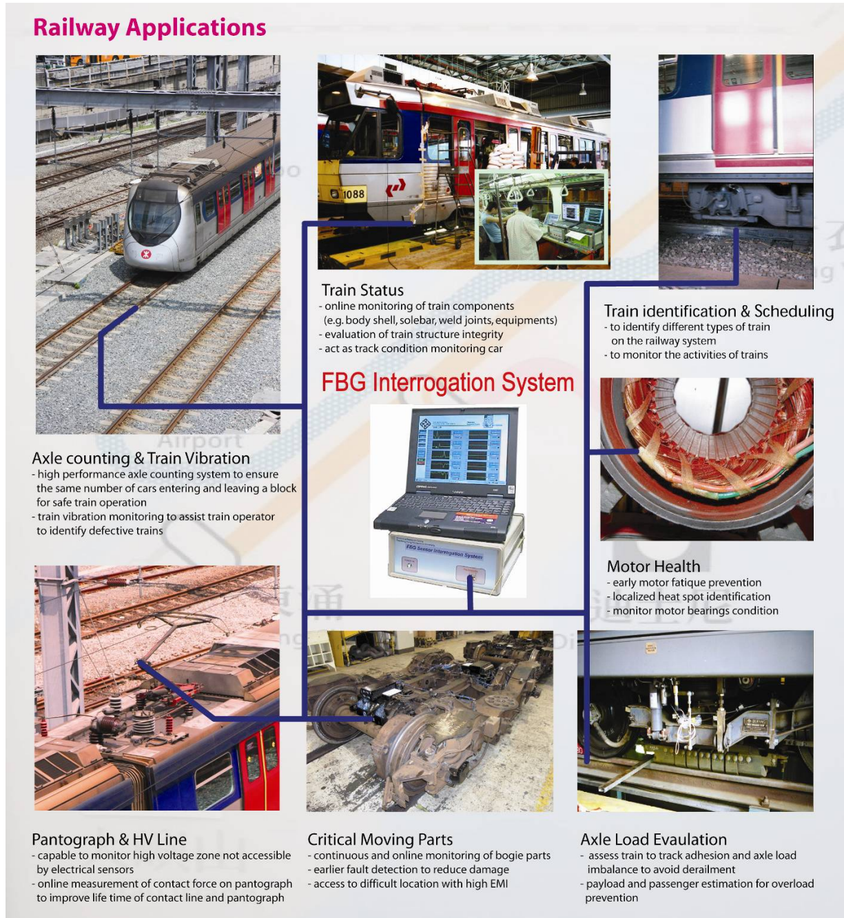
Figure 5: Many railway applications currently monitored using various conventional electrical sensor systems as shown in the figure could be replaced with FBG sensor technology.
