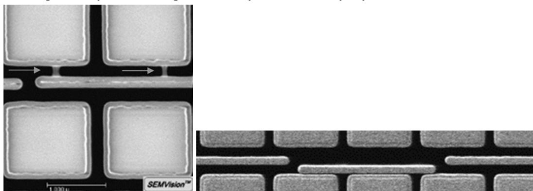
Figure 7: Watermarks in DT (left) & pattern collapse of silicon features (right)
