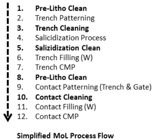
Figure 1.b: Figure showing a simplified Middle of Line (MoL) process flow.
